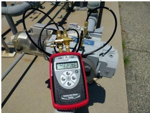
Figure 5: Differential pressure test using pete's plug
