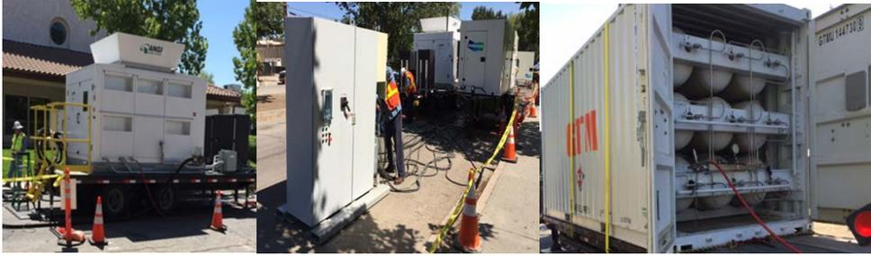
Figure 3: CNG Capture portable generator, mobile compressor, and CNG trailer<sup>60</sup>
