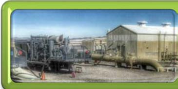
Pressure Reduction Using Mobile Compressors-common
